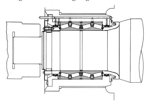
Bearings used in this application must have high radial and axial load carrying capacity. Therefore, NSK KV type, four roll tapered roller bearings and in some mills, NSK KH type, two roll tapered roller bearings are used. Special heavy duty roller retainer designs are used because of the high axial forces and misalignment. Low radial internal clearance insures that there is even load distribution across the bearing. Loose fits are used on both the inner and outer rings.
