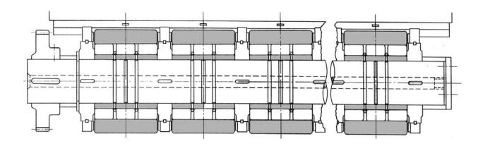
High running accuracy and careful matching of sets are an important feature for these bearings. The type of rolling element and the number of rows of rolling elements varies, but three rows of cylindrical rollers, NSK 3PLxxx type, is common. The inner rings are stationary on the shaft while the outer rings function as back-up rolls. Oil is supplied through the shaft to lubricate the bearings.
