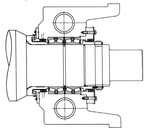
Workrolls in 4 high rolling mills use four row tapered roller bearings, NSK KV type. These bearings are slightly larger in size than those found in cold mills and also offers high capacity in both the radial and axial directions. The bearings are designed to be used with grease, oil mist, or oil-air system. Both the inner and outer rings are loose fitted.
