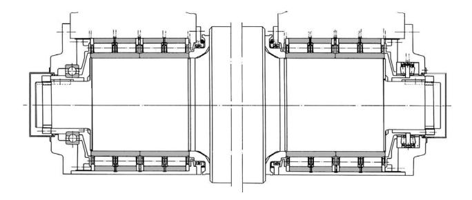
Four-row cylindrical roller bearings, **NSK RV** type, provide high load capacity necessary to support rolling loads while maintaining good accuracy. The inner rings are tight fitted to the rolls and are interchangeable from one bearing to another. A two-row tapered roller thrust bearing supports axial loads and a large ball bearing unitizes the drive side chock.
