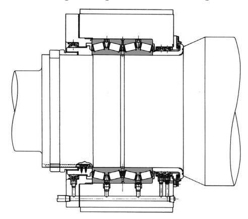
Large four-row tapered roller bearings, NSK KV type, are the most common bearings for work rolls in slabbery mills. Their ability to support high radial loads combined with axial loads make them a perfect choice. They have a loose fit with the roll and the housing and may be lubricated using grease, oil mist or oil-air systems.
