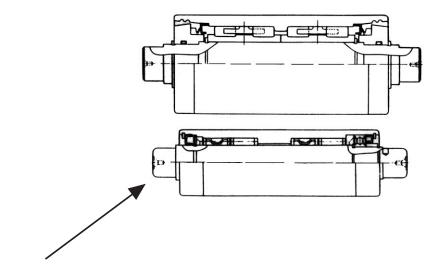
Backup Roll Units – Backup rolls offer high radial load capacity and are matched in sets to assure even support by all rolls. Optional special materials extend roll surface life in wet applications. Life of the assembly can be extended by using NSK regrind service.
