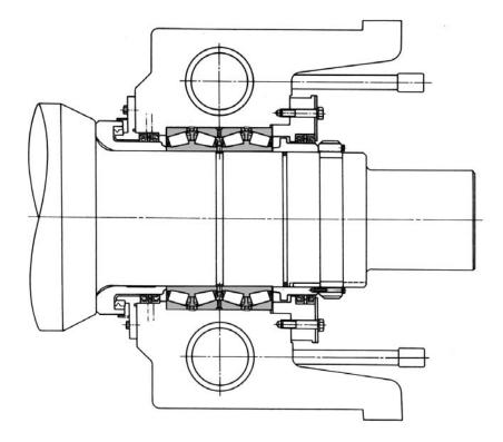
Most workrolls in a 4 high rolling mills use four row tapered roller bearings, NSK KV type. This bearing offers high capacity in both the radial and axial directions. The bearings are designed to be used with grease, oil mist, or oil-air system. Both the inner and outer rings are loose fitted. The intermediate roll of the modern 6 high mills also use this bearing.
