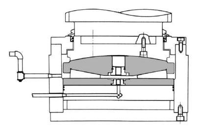
These high capacity tapered roller thrust bearings, NSK TFX type, sits on top of the top back up roll chock and is subjected to the hundreds of tons of rolling force. The spherical surface on the top race compensates for the misalignment created by the heavy load. Drip feed oil is used to lubricate these bearings.
