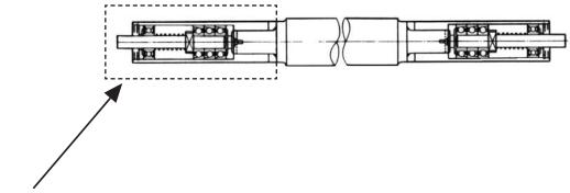
Thrust Blocks for Work Rolls and Intermediate Rolls – An assembly using angular contact ball bearings provides high thrust capacity and an ability to accelerate instantly. Low torque grease and seals provide reliable, maintenance-free operation.
