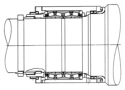
The NSK Sealed Clean Rollneck Bearings, KVE type, have replaced the conventional workroll bearings in many mills. Because they are sealed, they are better protected from rolling coolant and scale. Grease is packed in the bearings at installation and no further greasing is required for several months. This cuts operating costs substantially.
