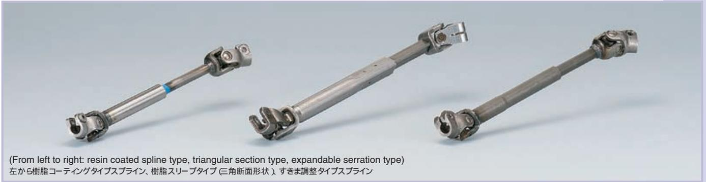
(From left to right: resin coated spline type, triangular section type, expandable serration type)
