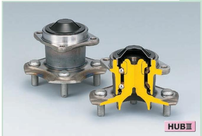
**Double-Row Angular Contact Ball Bearings with Inner and Outer Mounting Flange (HUB III for Non-Driven Wheels)**
