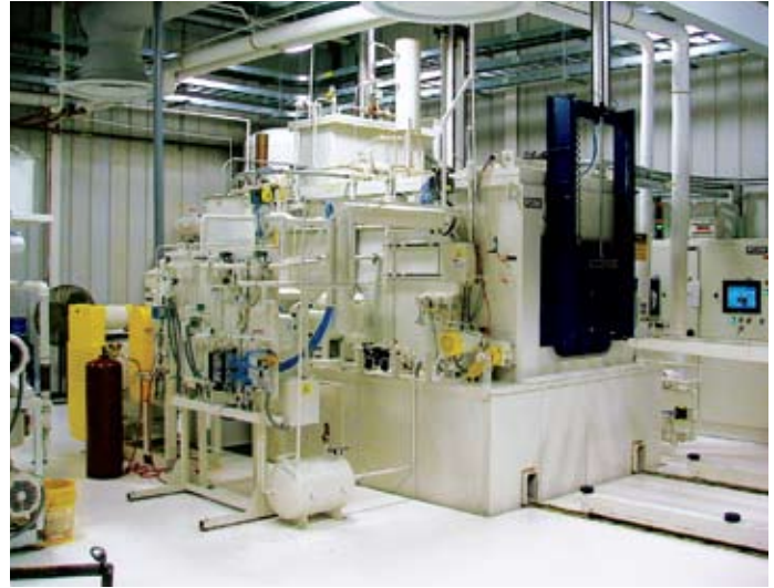
NHBB's vacuum carburizing furnace.
