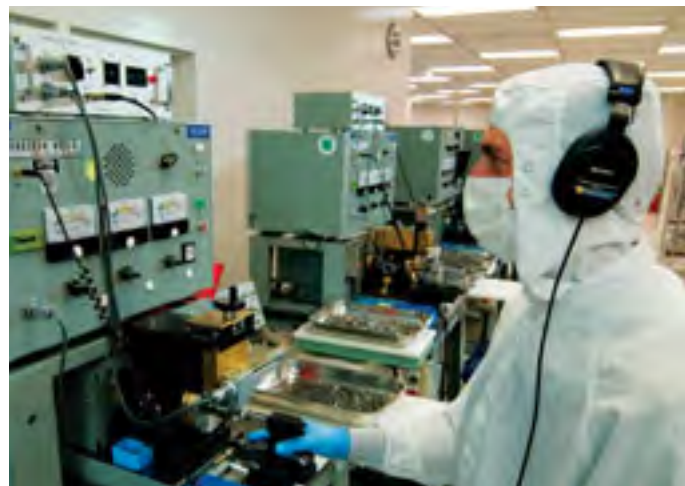
Anderometer, Dynamic Noise and Vibration Tester
