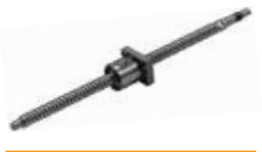
#BS25 Precision Ball Screws – Shaft Dia. 25, Lead 5, 10, 20
