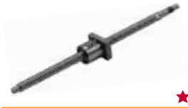
#BS20 Precision Ball Screws – Shaft Dia. 20, Lead 5, 10, 20
