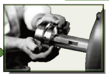
**Shaft spacing** should be within range given by dimensions 'W' and 'X' as shown in charts on page 4. **Position each hub** on proper size shaft - Magnaloy couplings are bored to standard "push fit" tolerances, if a tight fit exists, check shaft for burrs.
