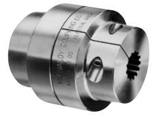
**The Clamp-Type Coupling** utilized the basic Magnaloy coupling with the addition of the clamp feature. Developed to compensate for variations in spline formation methods and tolerances. Assures centering of the coupling and positive retention on the shaft. The clamp feature is suggested for all splined couplings, but is also available in smooth bored and keyed models.
