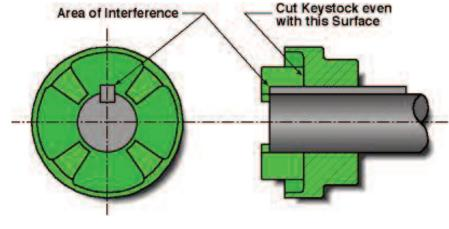
Failure to correct this condition will result in assembly difficulty and could cause damage to the drive or driven equipment. Check our web site at www.magnaloy.com for other bulletins.
