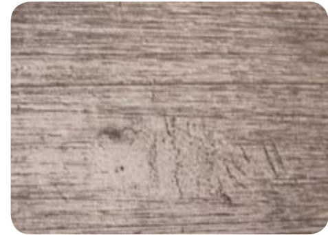
Wear caused by static vibration
