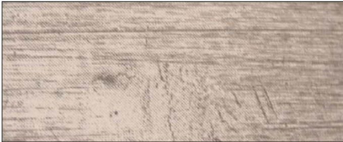
Wear caused by static vibration
