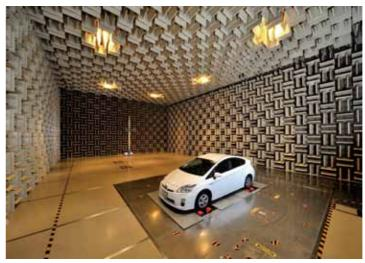
Electromagnetic Anechoic Chamber
