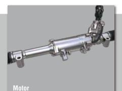
Layout with rack and motor on the same axle realizes direct-response feel
