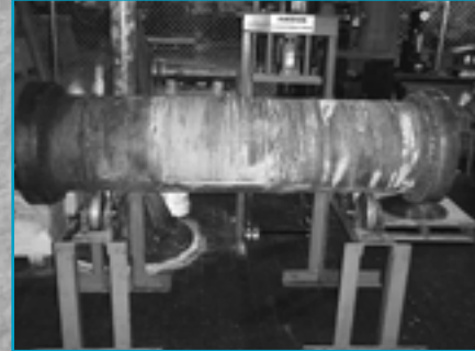
LM 2500 gas turbine coupling before being refurbished
