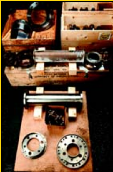
High performance coupling for refurbishment
