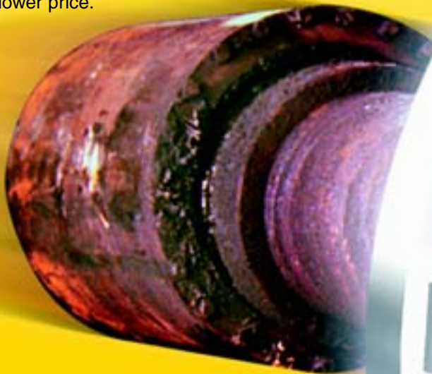
A universal joint, as received from a customer, at our service center for inspection and rebuilding
