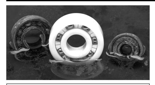
STEEL BEARINGS CORRODE IN LIQUIDS
