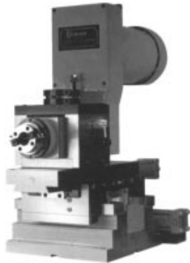
9 18084 Three axis milling unit consisting of a hardened way slide, dovetail slide and a special vertical travel unit featuring a Model 3500 #30 N.M.T.B. nose spindle.
