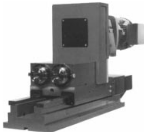
11 17745 Dual motorized spindle unit featuring (2) Model 4000 spindles with #40 N.M.T.B. nose, and powered by an AC gearmotor and timing belt mounted on a HWS12 slide.
