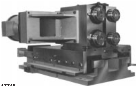
10 17748 Four spindle cluster mounted on a HWL12 slide. The cluster unit consists of (2) Model 3500 and (2) Model 2750 boring nose spindles with AC motors and poly-V belt drives. Designed to allow for variable spindle center-to-center distances.
