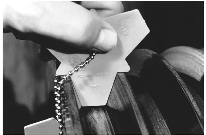
Pulley gauges make wear detection easier.
