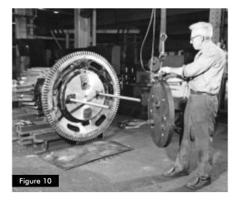
5. For hubs without puller holes, drill and tap two holes in the hub to receive the threaded stud bolts, Figure 10. Assemble the alloy tool steel plate on the threaded stud bolts as shown in Figure 11. Refer to Tables 1 thru 8 for a listing of Falk recommended puller bolt hole sizes.
