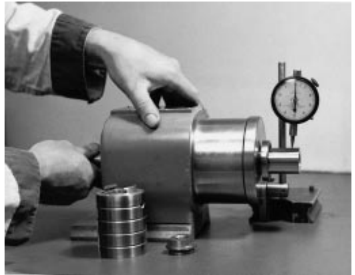
Figure 6 – Checking Nose-End Runout
