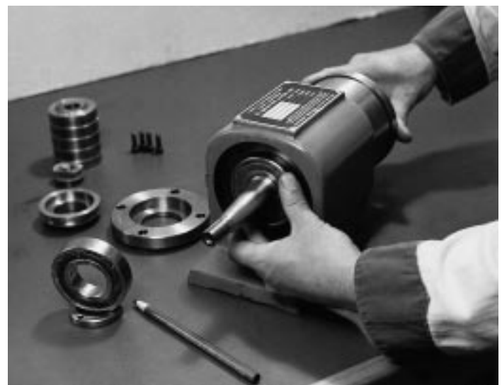
FIGURE 5 – MOUNTING DRIVE-END BEARINGS
