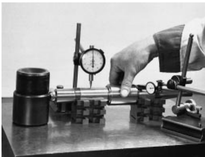
Figure 2 – Inspection of Shaft
