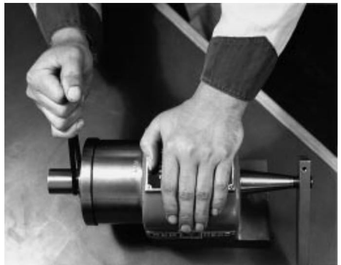
Figure 7 – Tightening with Spanner Wrench
