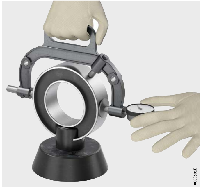
Figure 10 Setting the snap gauge by means of the master ring
