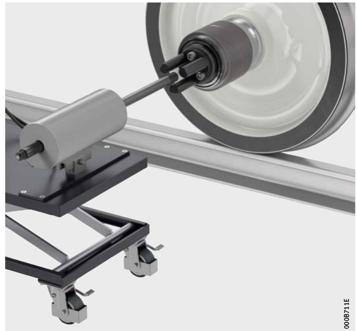
Figure 4 Inserting the spindle through the hollow piston
