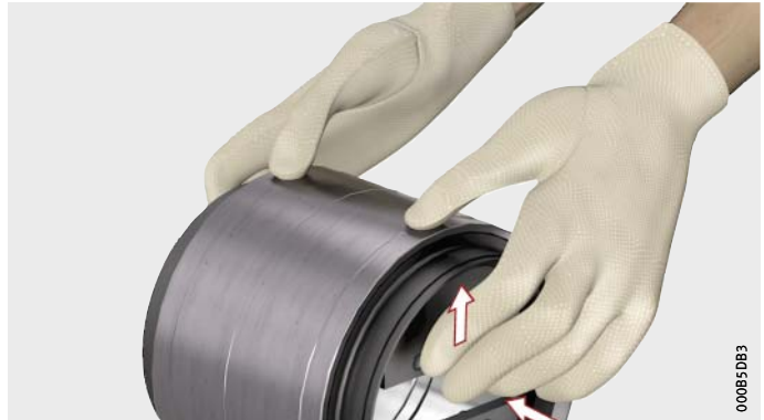
Figure 10 Inserting the press-out segments
