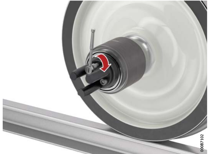
Figure 3 Screwing on the guide bush
