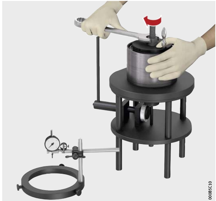
Figure 9 Tightening the nut using a wrench
