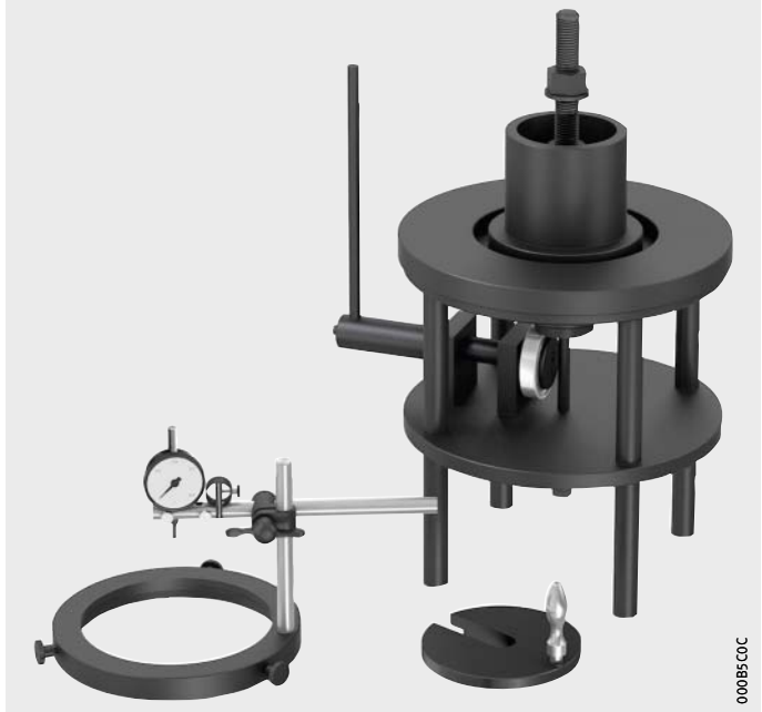
Figure 7 Fitting the centring bush
