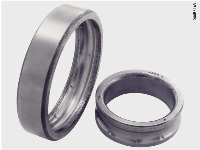
Figure 2 Rolling element indentations (brinelling)
