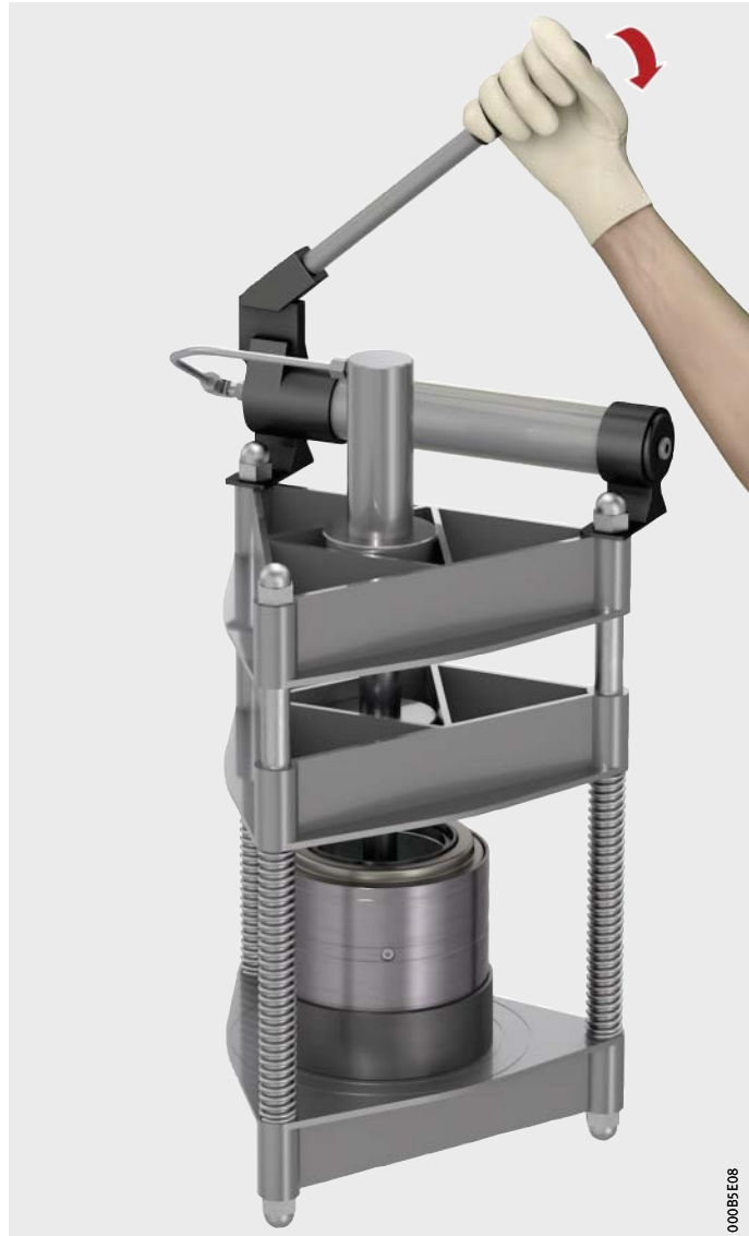
Figure 19 Inserting the TAROL unit in the plate press, aligning the unit and activating the press
