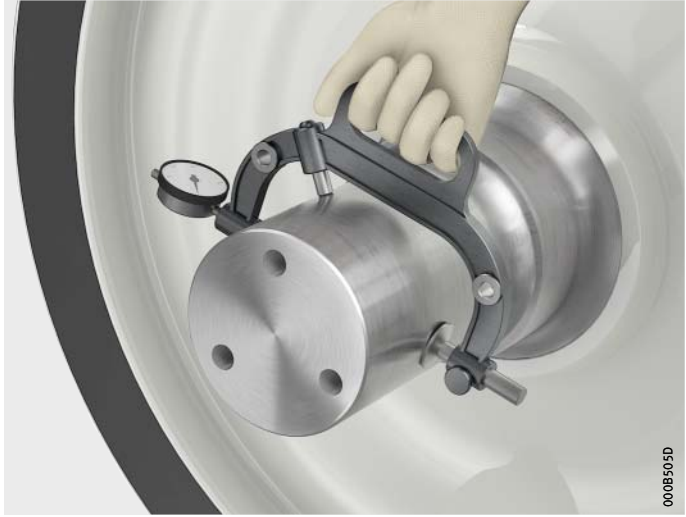
Figure 11 Measuring the shaft journal using the snap gauge
