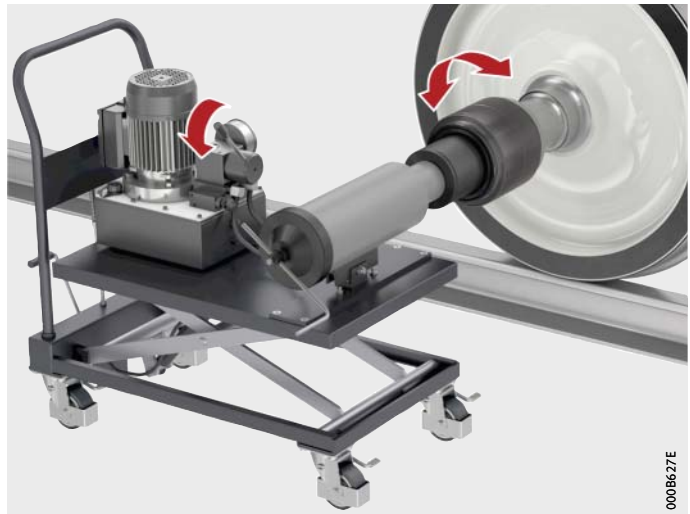
Figure 7 Pressing the bearing unit into place
