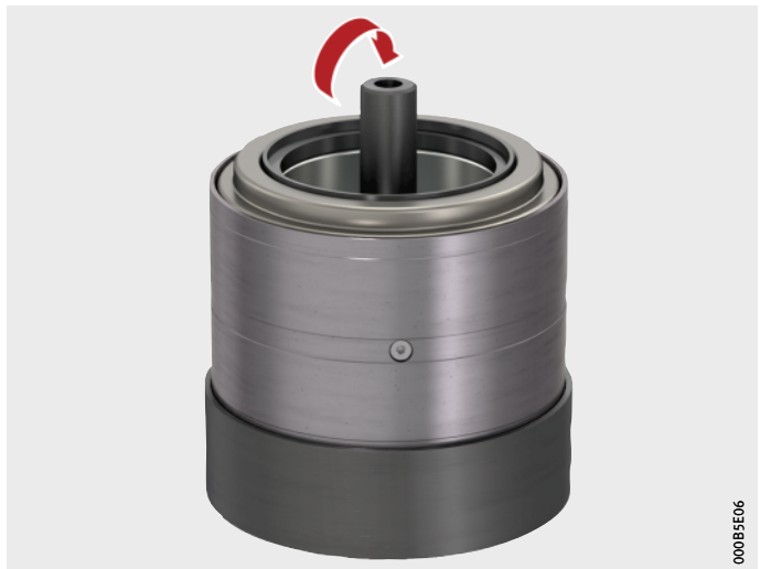
Figure 18 TAROL unit with press-out tool in locating ring and punch with punch plate
