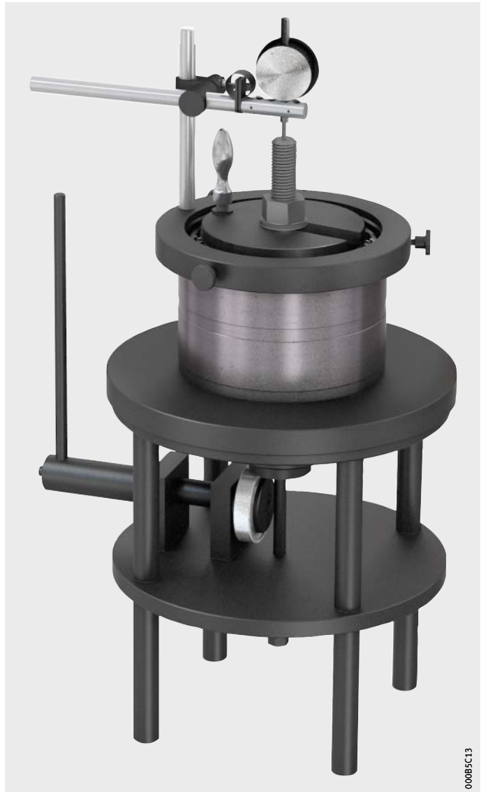
Figure 11 Locating ring with dial gauge
