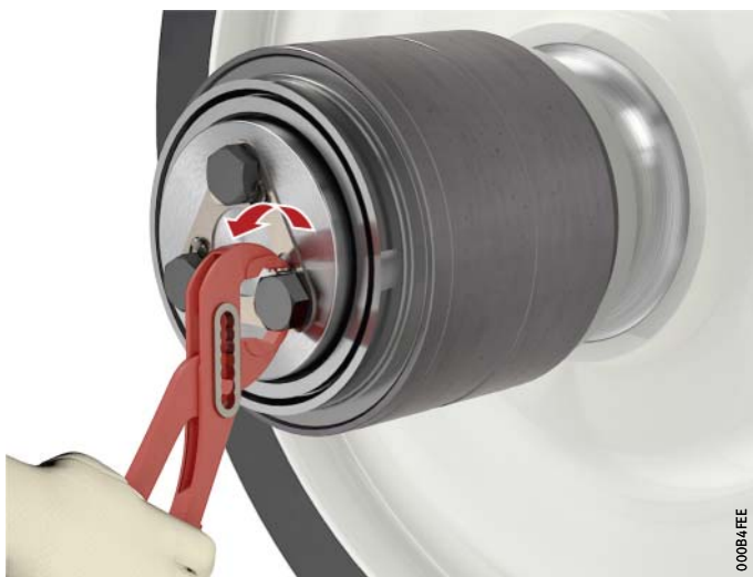
Figure 10 Bending back the tab on the tab washer
