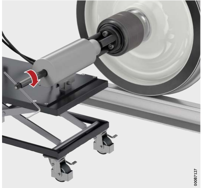
Figure 5 Screwing the spindle into the guide bush
