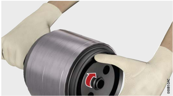
Figure 12 Axially tensioning the punch and segments
