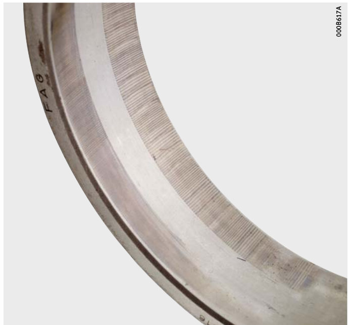
Figure 5 Current passage damage
