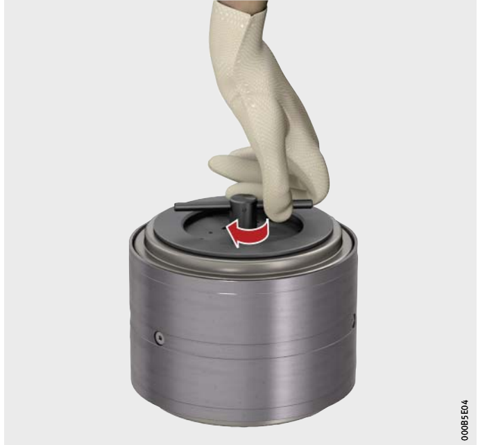
Figure 17 Positioning and tensioning the press-out tool on the TAROL unit
