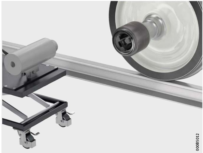
Figure 3 Moving the hydraulic unit into place
