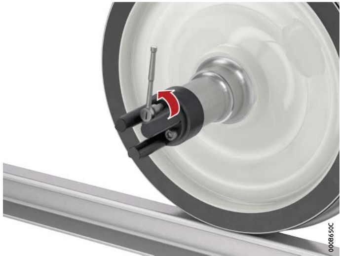
Figure 7 Unscrewing the guide bush
