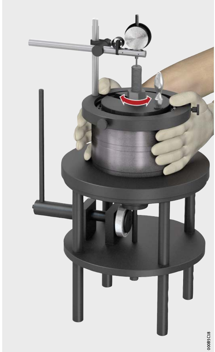
Figure 12 Rotating the outer ring
