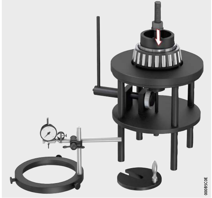
Figure 8 Sliding the inner ring onto the centring bush
