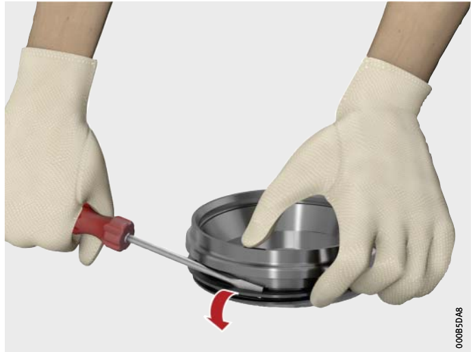
Figure 20 Removing the lamellar rings
