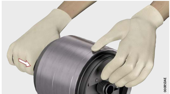
Figure 11 Guiding the punch through the bearing bore
