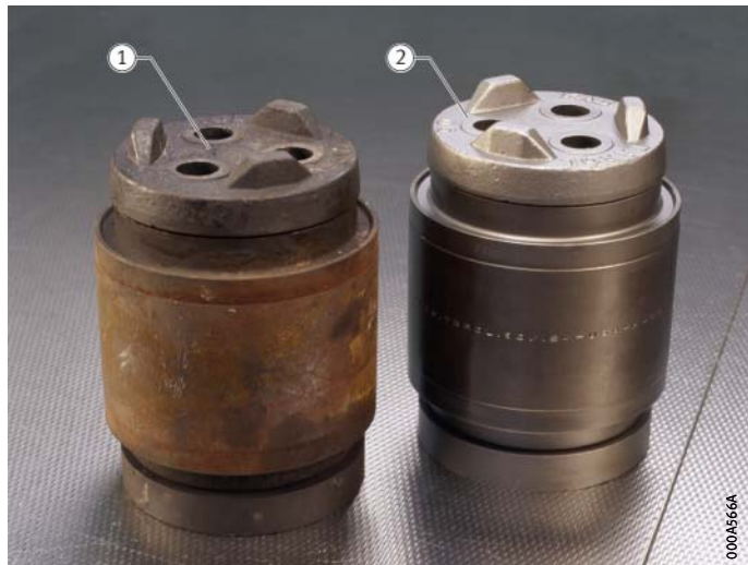
① Before reconditioning ② After reconditioning
