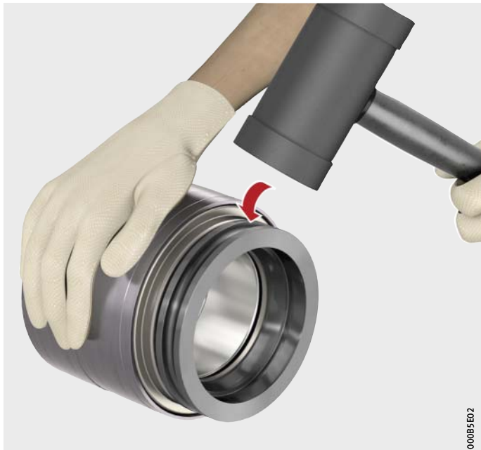
Figure 16 Removing the backing ring in the TAROL variant with the sheet metal cap seal
