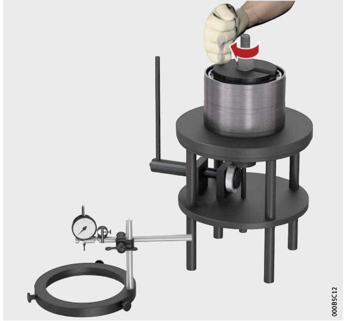
Figure 10 Rotating the outer ring
