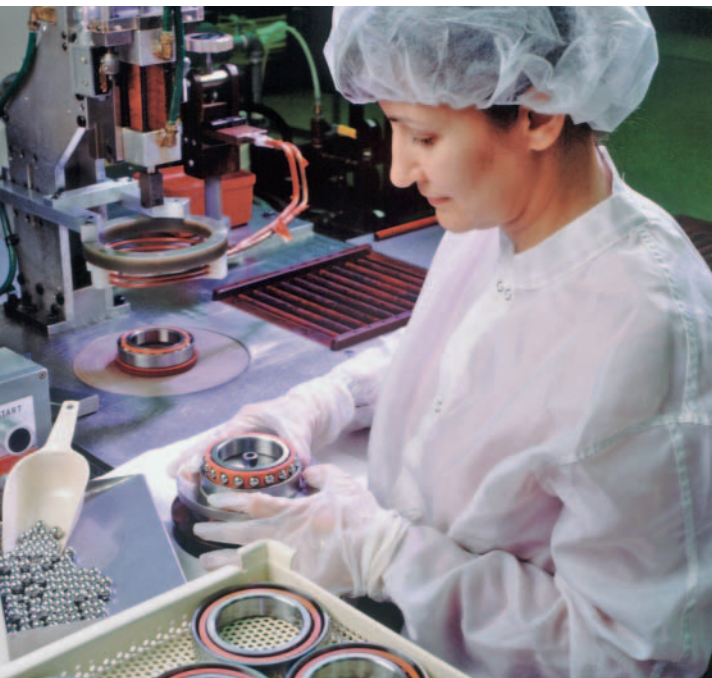
... in bearing assembly
