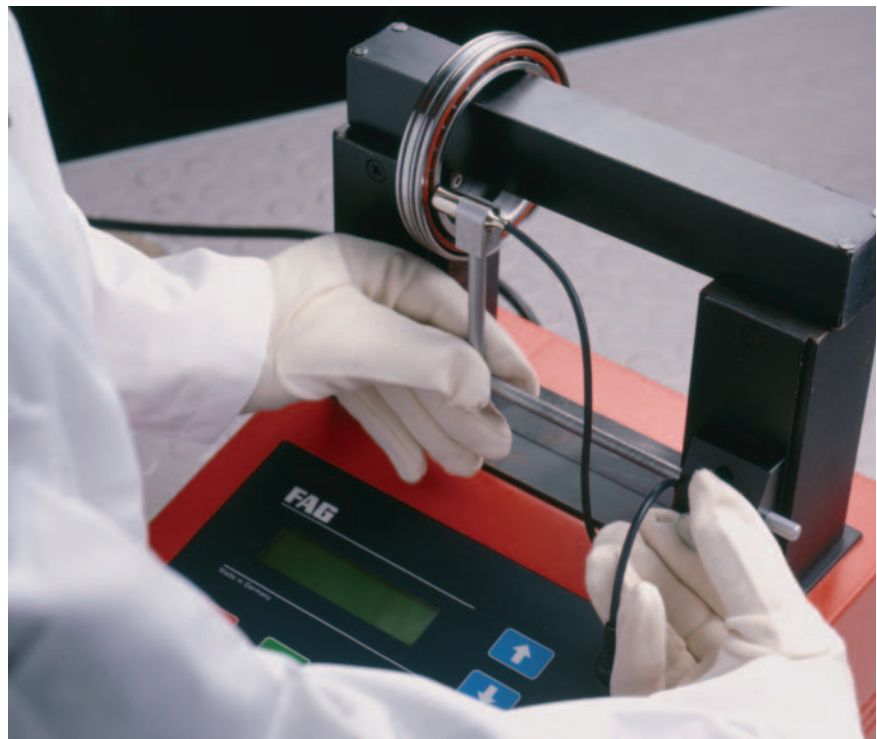
3: Warming a spindle bearing using an inductive heating device
