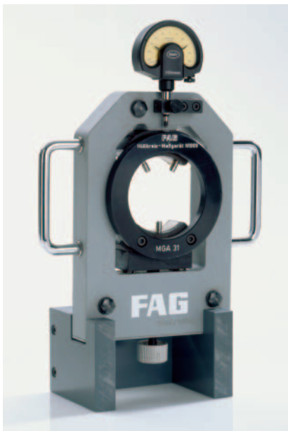
15: FAG enveloping circle gauge MGA 31 for setting radial internal clearance of cylindrical roller bearings with removable inner ring
