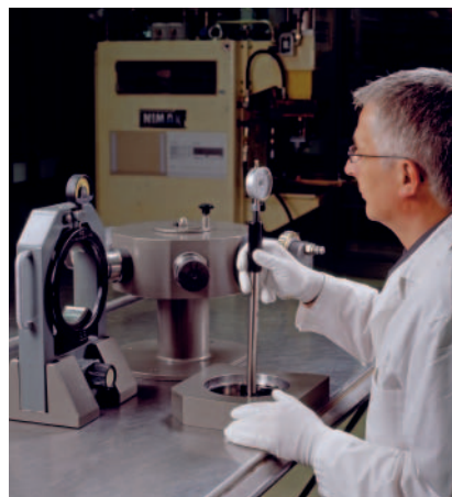
9: Determination of outer ring raceway diameter
