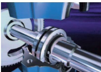
6 Lower the shaft in order to subject the bearing to load
