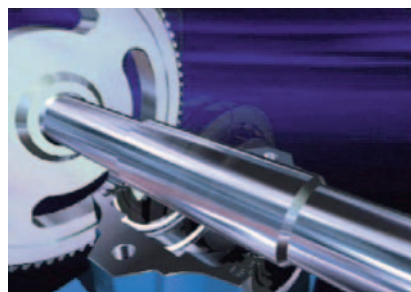
4 Place the outer ring half in the lower section of the housing and align it with the inner ring mounted on the shaft, then screw together the inner ring halves
