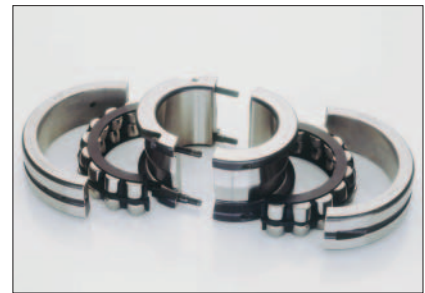
4: Split spherical roller bearing with split solid cage made from glass fibre reinforced polyamide or brass, with integral locking rings
