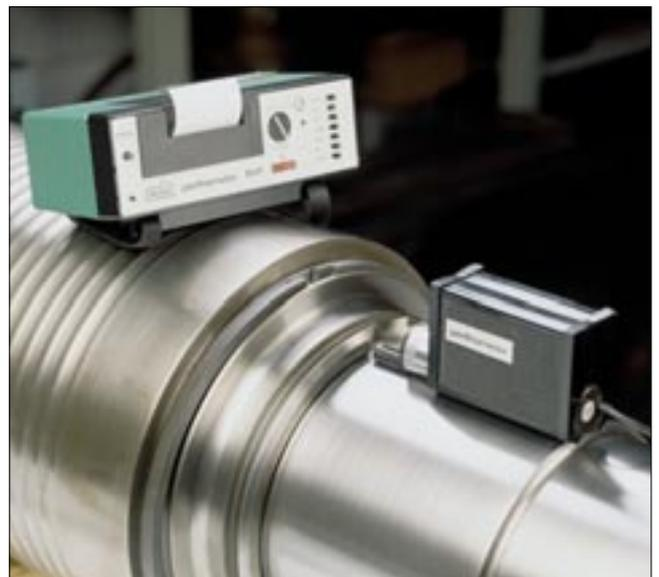
67: Checking the surface roughness
