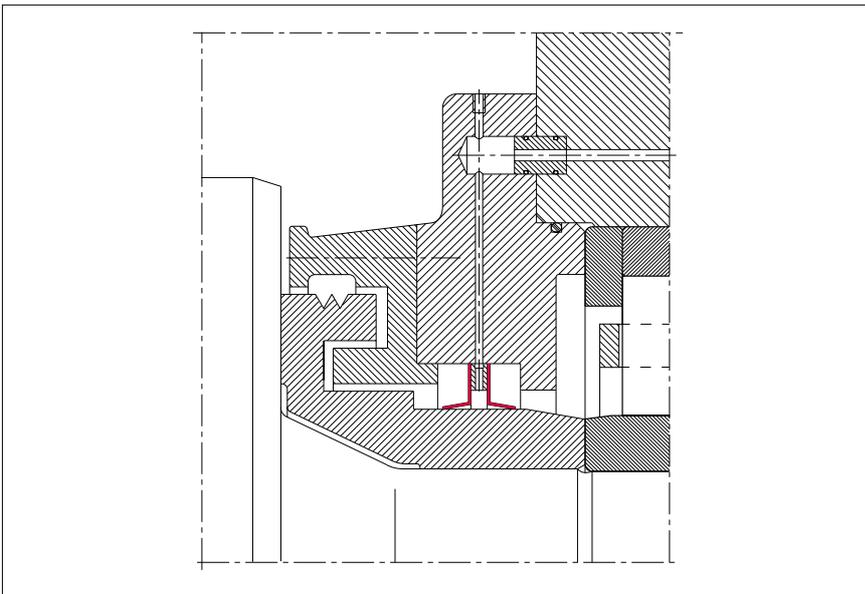
59: In cold-rolling stands the sealing lip of the inner collar seal must be directed towards the bearing (back-up roll)
