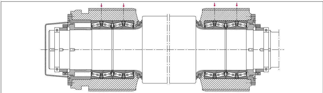
b) Roll neck bearing arrangement with four-row tapered roller bearings
