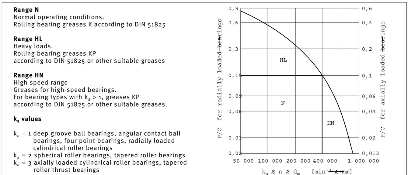
42: Grease selection from the load ratio  $P/C$  and the relevant bearing speed index  $k_a \times n \times d_m$
