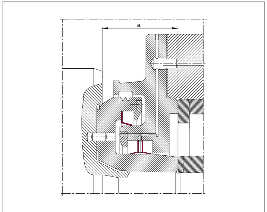
55: Sealing for large hot-rolling stands exposed to heavy contamination
