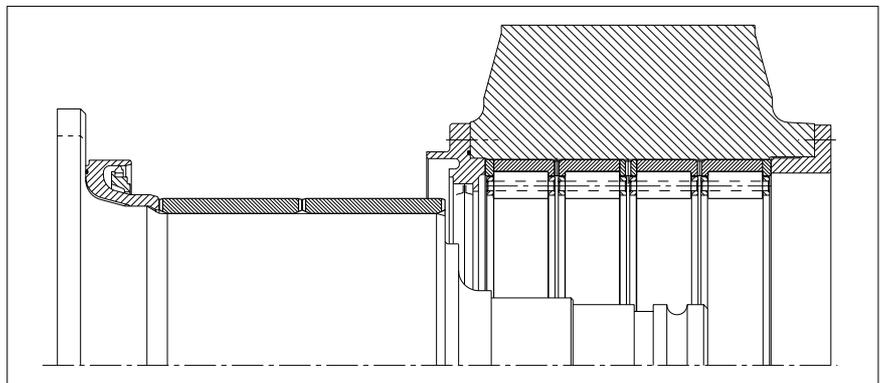
77: The pre-assembled chock is pushed onto the roll neck.
