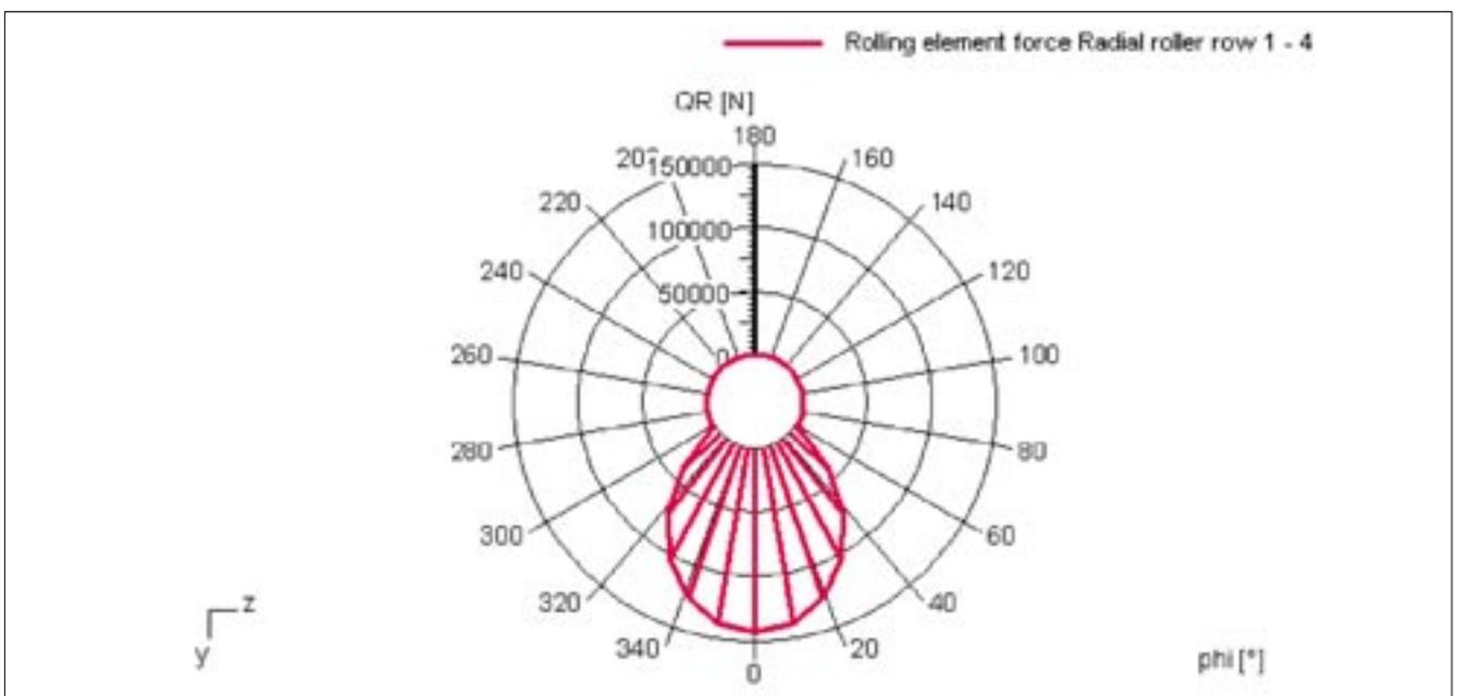
z8b: Load distribution within the four-row cylindrical roller bearing on the back-up roll
