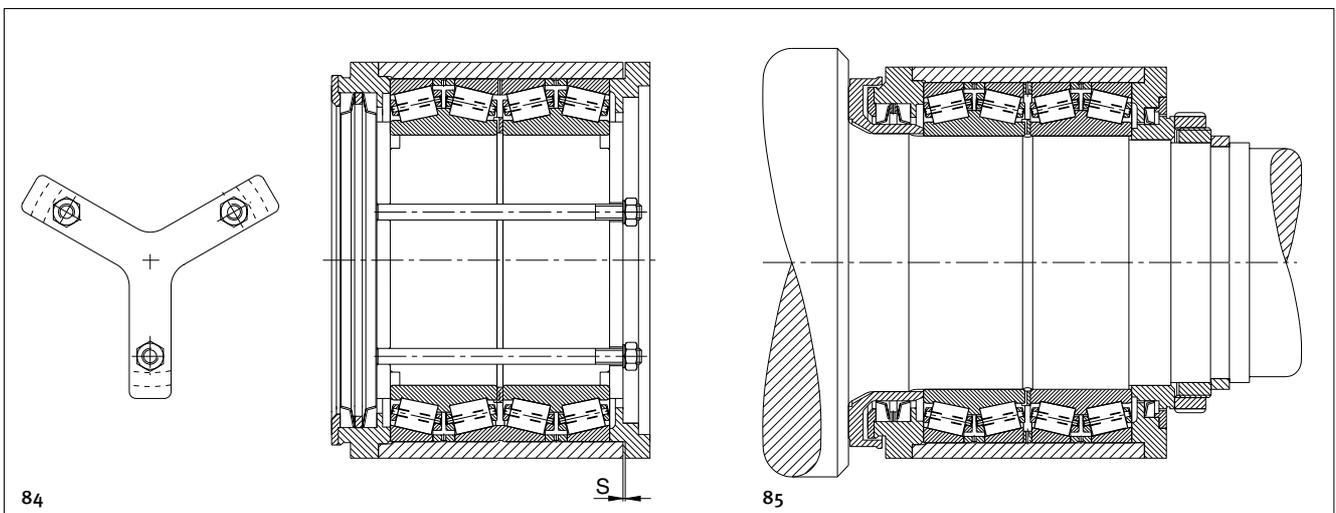
84: The cups are clamped together while the cones are constantly rotated.
