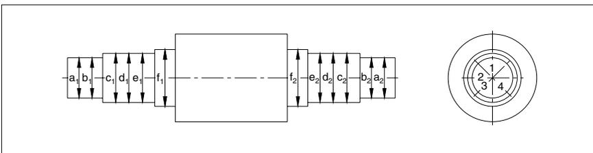
61: Measuring points for checking roll necks
