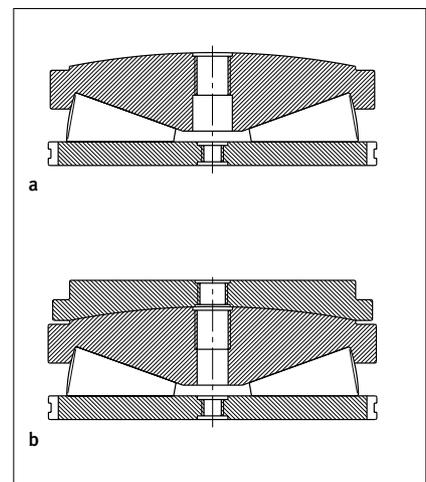
18: Tapered roller thrust bearings for screw-down mechanisms
