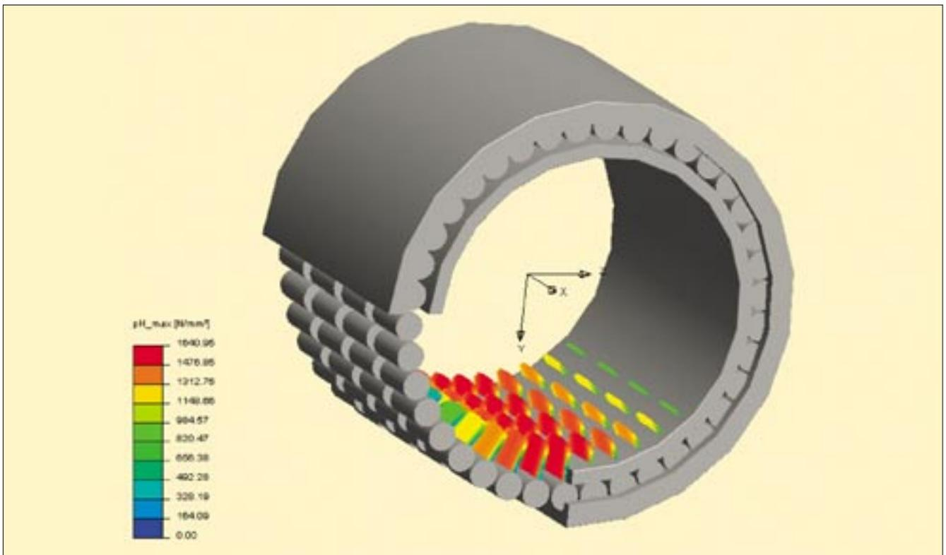
z8a: Visualisation of the pressures acting on the four-row cylindrical roller bearing on the back-up roll
