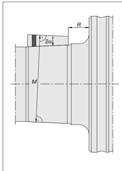
63a: Straight edge of the FAG Taper Measuring Instrument MGK9205
