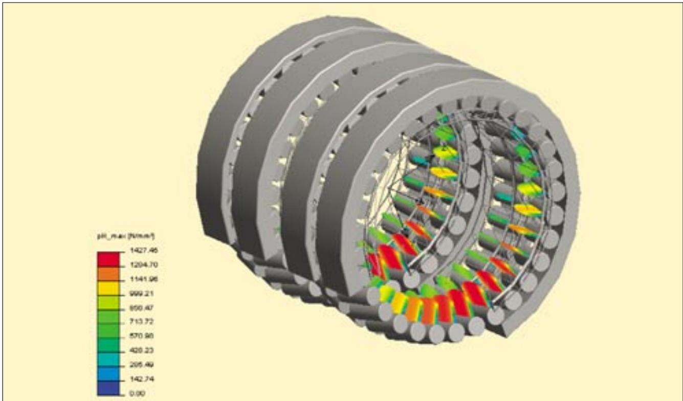
29a: Visualisation of the pressures acting on the four-row tapered roller bearing on the work roll
