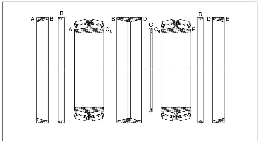
80: Sequence of assembly of the bearing components
