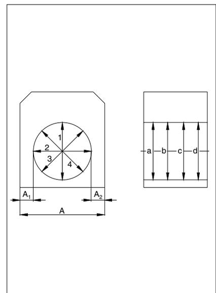
64: Measuring points for checking the chock
