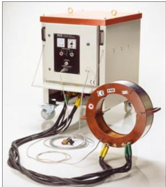
88: FAG low-voltage induction coil with transformer
