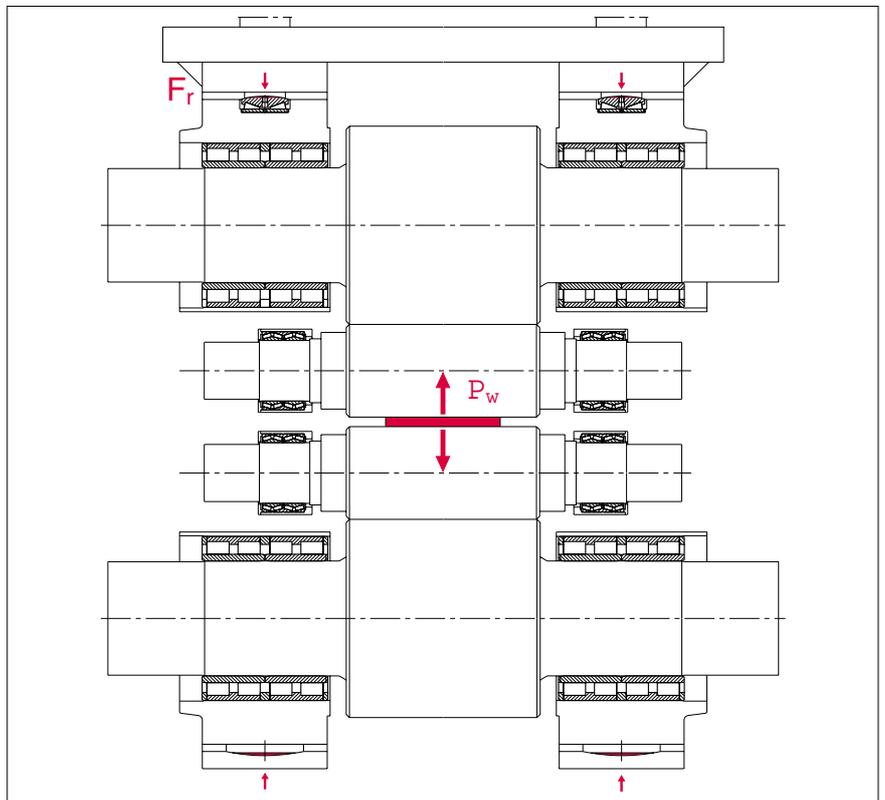
20: Self-aligning chocks for strip rolling
