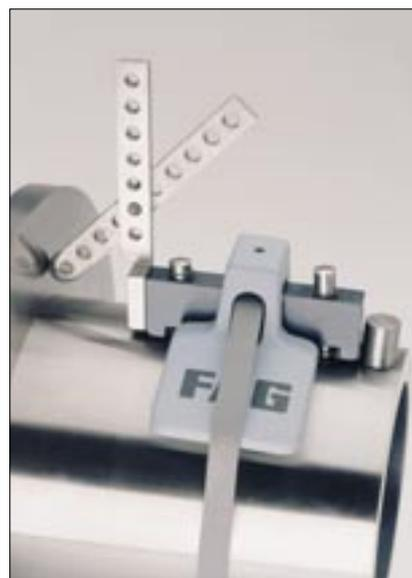
63b: Measuring a tapered roll neck with an FAG Taper Measuring Instrument MGK9205; the stop touches the front datum surface.
