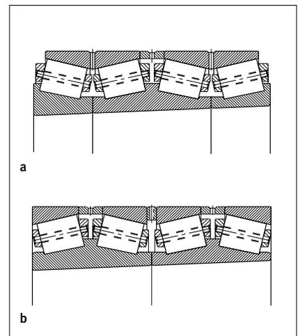
13: Four-row tapered roller bearing with tapered bore and pin-type cage
