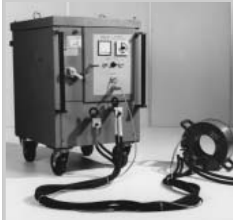
▼ Heating rings are suitable for dismantling the inner rings of cylindrical roller bearings
