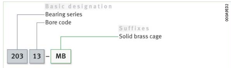
4 Barrel roller bearing with cylindrical bore: designation structure
