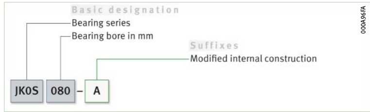
16 Integral tapered roller bearing: designation structure
