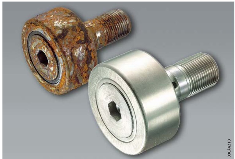
Uncoated and coated stud type track roller in the salt spray test
