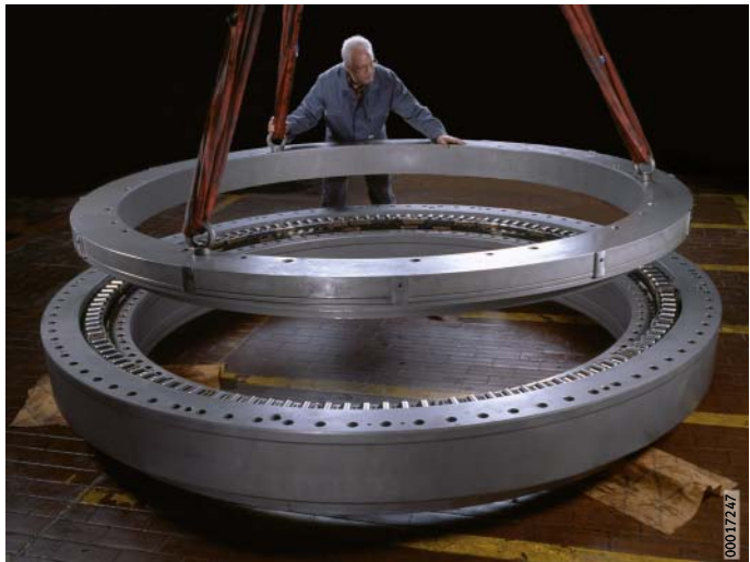
Figure 9 Mounting of a new rolling bearing ring
