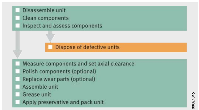
Figure 2 Reconditioning of TAROL units
