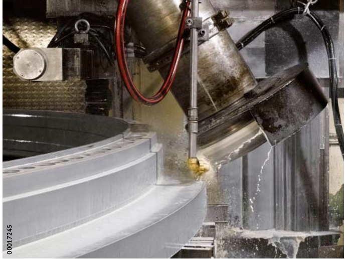
Figure 7 Regrinding of large size bearing ring
