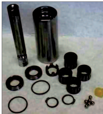
10: Components of a leveller for a strip mill
