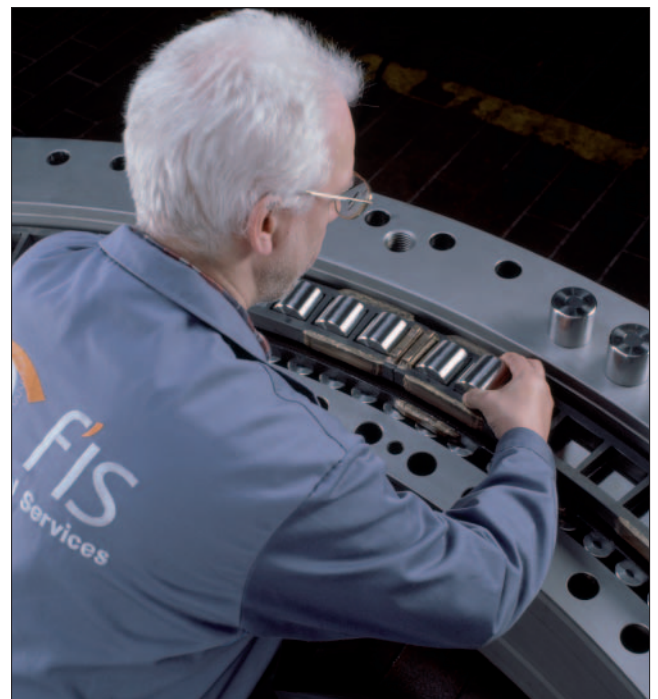
2: Mounting of a reconditioned tunnel boring machine bearing
