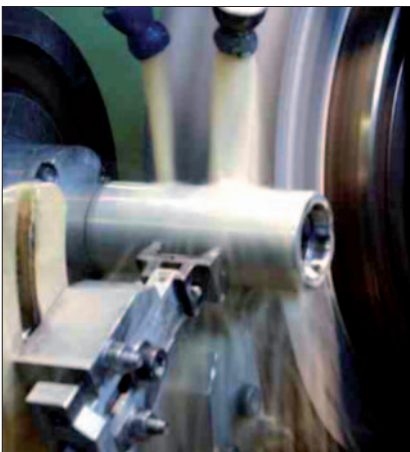
9: Grinding of a leveller unit
