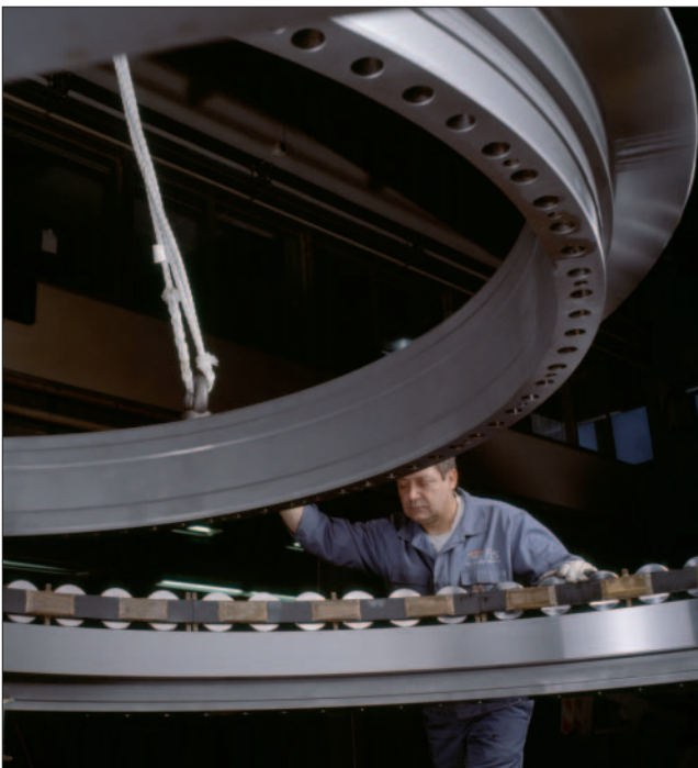
1: Mounting of a reconditioned tunnel boring machine bearing
