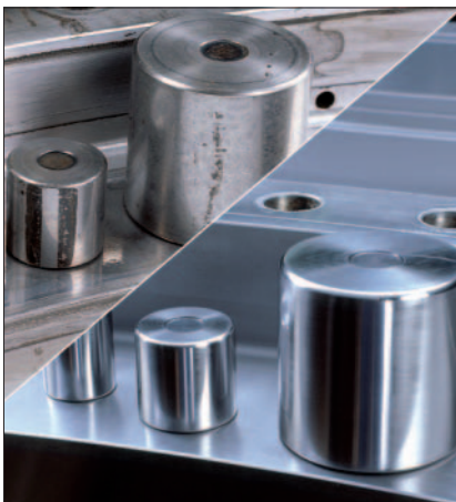
6: Before: Rollers with corrosion marks and foreign body indentations After: New rollers with matched oversize
