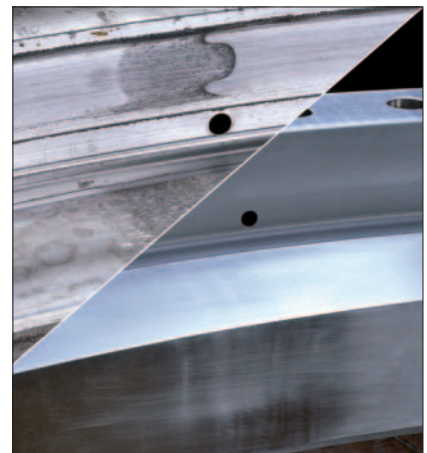
8: Before: Raceway with heavy scar formation in the area of the slippage point After: Reground raceway
