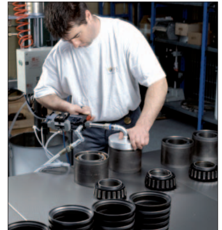
5: Greasing of TAROL units
