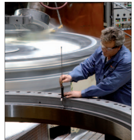
11: Regrinding and inspection measurement of a large rolling bearing ring
