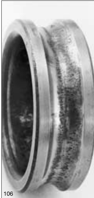
106: Flaked inner ring of a deep groove ball bearing
