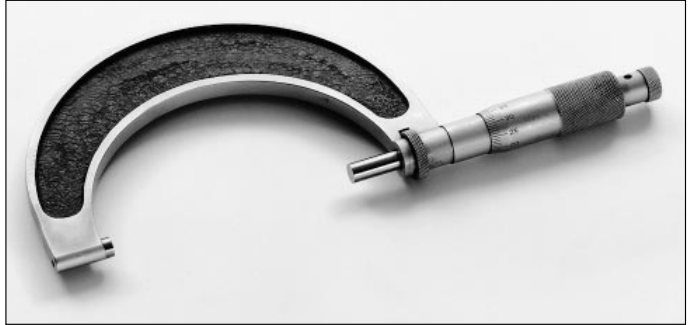
2: External micrometer for measuring shaft diameters
