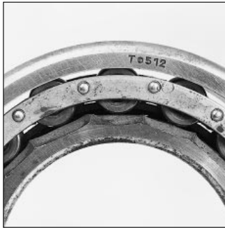
111: Fractured lip of a barrel roller bearing inner ring driven up its seat by hammer blows
