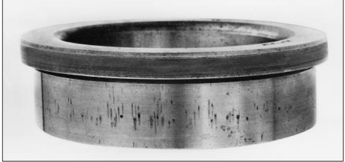
109: Scored raceway of a cylindrical roller bearing inner ring
