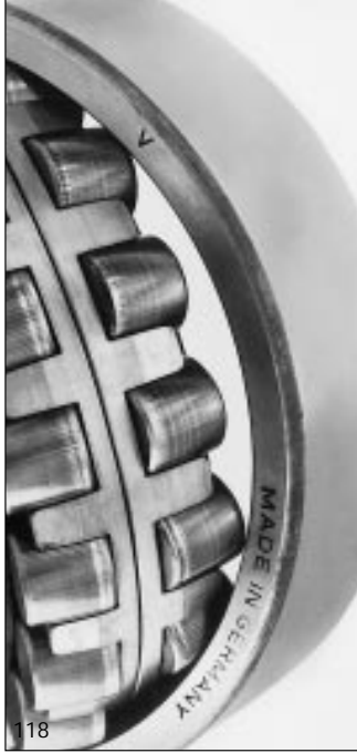
119: Fluted raceway of a spherical roller bearing outer ring due to the passage of electric current
