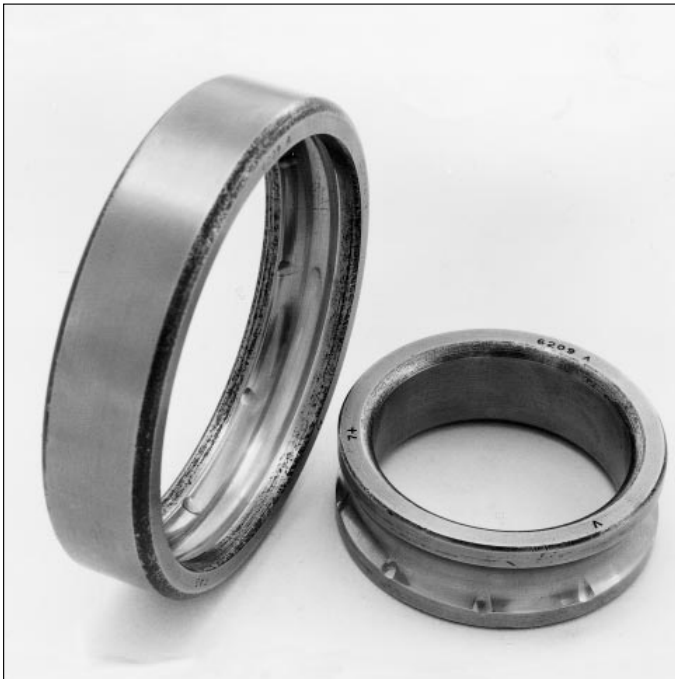
108: Ball indentations in the raceway of a deep groove ball bearing resulting from faulty mounting
