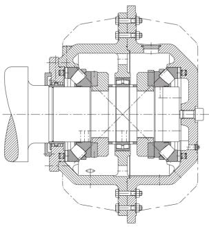
63b: Ship shaft thrust block with FKA flanged housing
