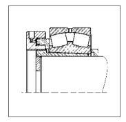
94: Hydraulic nut for dismounting a withdrawal sleeve mounted spherical roller bearing. The projecting portion of the sleeve is backed up by a thick-walled support ring.
