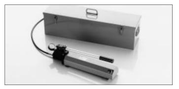
52: Hand pump set FAG 173746, consisting of a two-step piston pump (800 bar) with 3-litre oil container, manometer, extreme pressure hose and fitting (connecting thread G 1/4)
