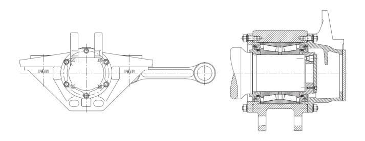
46: Axle box roller bearings of the ICE driving unit
