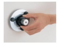
f: series 562: tighten both threaded pins.
