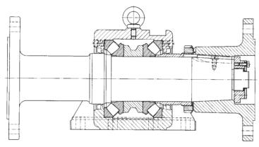
63a: Complete ship shaft thrust block FAG BEHT.DRL.110.1..... (SGA plummer block housing)
