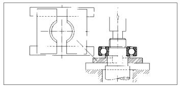
Provisionally, small bearings can be driven off their seat with a hammer and a metal drift (Fig. 84, right). The light hammer blows should be applied evenly round the whole circumference of the tight-fitted ring.
