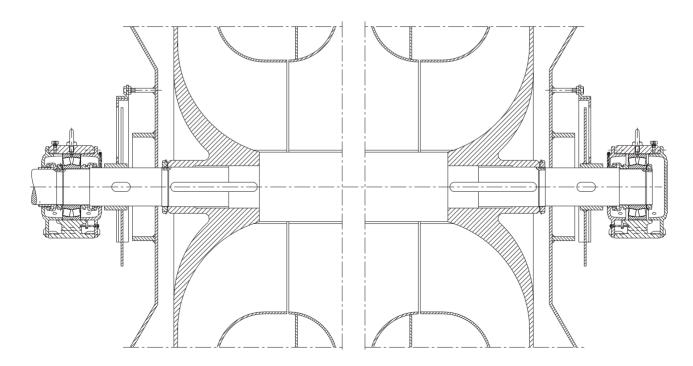
118: Rotor mounting of an exhauster
