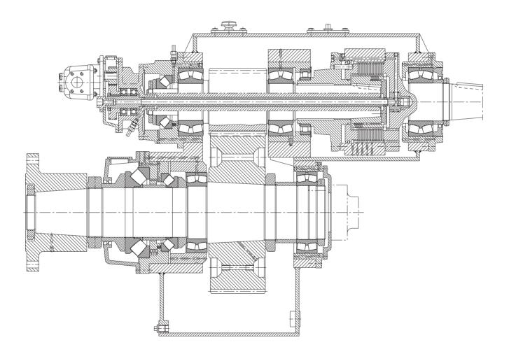
28: Bearing arrangement of a marine gear
