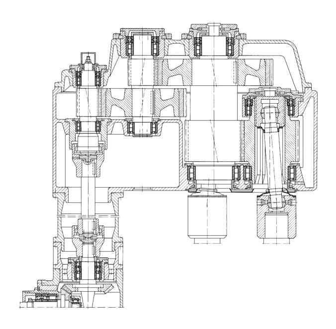
107: Combined reduction and cogging wheel gear of a billet mill
