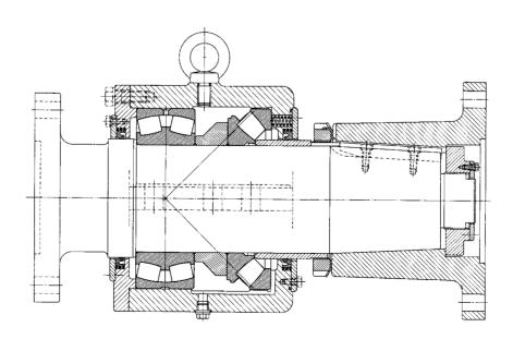
64b: Complete ship shaft thrust block FAG BEHT.DRL.200.1..... (SUB pot-shaped housing)
