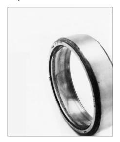
37: Development of tracks in the case of a self-aligning ball bearing with rotating inner ring under detrimental axial preload and radial load
