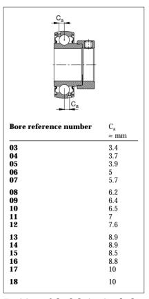
Position of the lubricating hole relative to the outer ring centre
