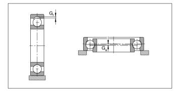
G<sub>r</sub> radial bearing clearance
