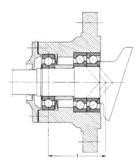
116: Drive flange of an axial piston machine
