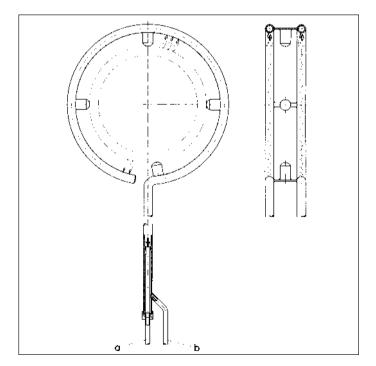
97: Ring burner for dismounting inner rings a = gas, b = air
