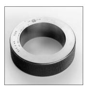
Master taper ring for checking small tapered bearing seats
