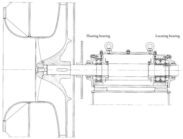
119: Rotor bearings of a hot gas ventilator
