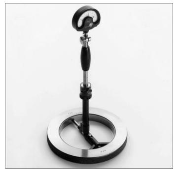
5: Comparative measuring instruments are especially suitable for bore measurements. The master ring is used for setting.
