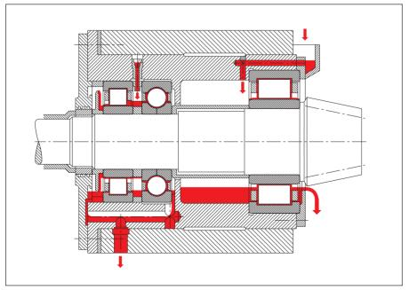
62: Oil jet lubrication with nozzles
