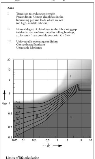
As is the case with the former life calculation method, only material fatigue is taken into consideration as a cause of failure for the *adjusted life calculation* as well. The calculated life can only correspond to the actual service life of the bearing when the lubricant service life or the life limited by wear is not shorter than the fatigue life.
