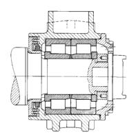
48: Axle box roller bearings for an underground train
