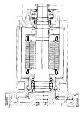
18: Bearing arrangement of a surface grinding spindle
