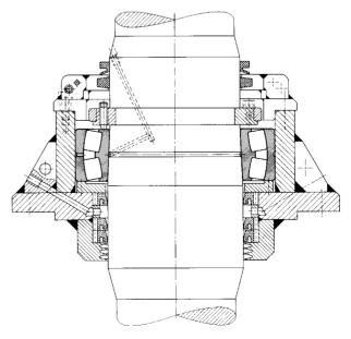
57: Rudder shaft bearing FAG RS3052KW.1.....
