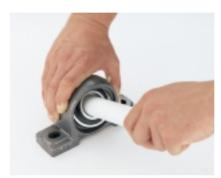
e: Manually tighten eccentric selflocking collar with a slight jerk in the direction of shaft rotation.
