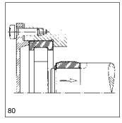
79: Start dismounting of nonseparable bearings with the loose-fitted ring.
