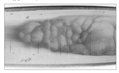
75: Slippage damage on the inner ring of a cylindrical roller bearing
