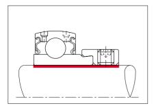
The bearings are fastened on the shaft either by means of eccentric self-locking collars or two threaded pins.
