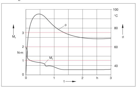
These effects are even more intensive, the larger the grease quantity in and beside the bearing and the more the movement of the grease out of the bearing is obstructed. They can be counteracted by an interval lubricant supply system with accordingly specified downtimes for cooling such as is used for spindle bearings in machine tools.
