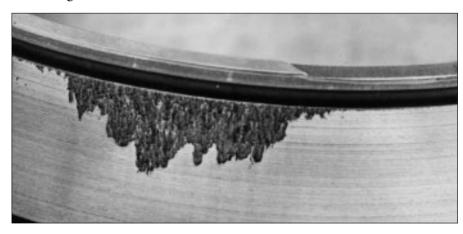
48: Fatigue at the raceway edge in the case of ball bearings, e.g. with high moment load (edge running); left raceway edge, right ball.
