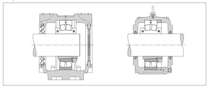
2: Easy to inspect, fast and easy mounting – the FAG split spherical roller bearing directly before mounting into an SNV housing.
