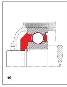
little grease remains in the bearing at the side facing the grease valve. This can be avoided by displacing the gap between the rotating grease valve and its stationary counter part nearer to the shaft. A normal grease valve where the gap is at bearing outer ring level (fig. 44a) has a strong
