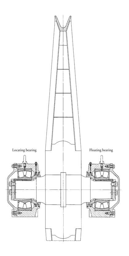
75: Rope sheave (underground mining)
