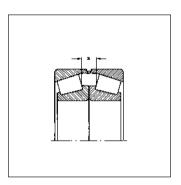
63: Double row tapered roller bearing in O arrangement
