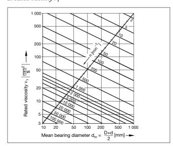
The basic a<sub>23II</sub> factor can be determined as a function of K on one of the curves in zone II by means of the value K (K = 0 to 6).
