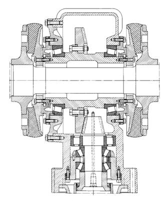
55: Bevel gear transmission for city trains
