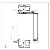
101: Bearing seated on withdrawal sleeve: Oil is pumped into withdrawal sleeve bore and O. D.; withdrawal sleeve disengages spontaneously. Nut to be left on shaft.
