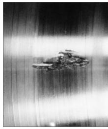
52: Failure mechanism as in fig. 51 but with wear of the raceway edges, cross profile of the roller see fig. 69.
