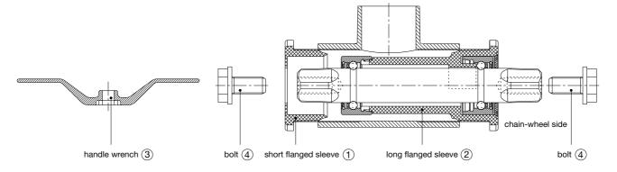
**Tool**The FAG WKZG.564414 ③ handle wrench is used for mounting and dismounting.
