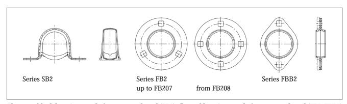
Plummer block housings made from pressed steel (SB2); flanged housings made from pressed steel (FB2, FBB2)
