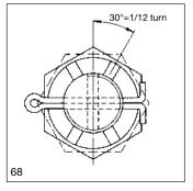
68: Tighten castle nut while rotating the wheel, until drag is felt.
