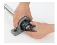
f: Localize eccentric self-locking collar by means of metal drift and hammer.
