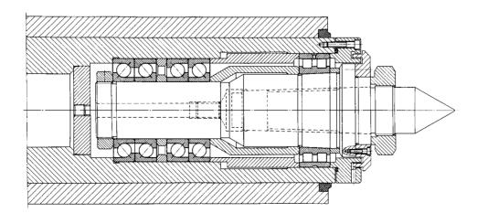
20: Bearing arrangement of a tailstock spindle
