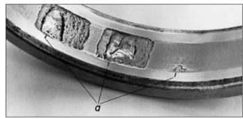
111: Fractured lip of a barrel roller bearing inner ring driven up its seat by hammer blows
