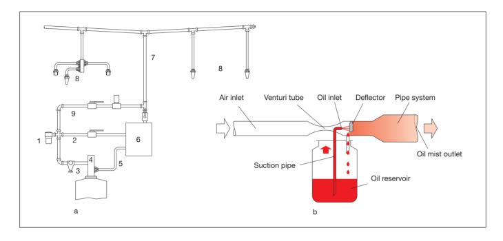
24a: Schematic drawing of an air-oil lubrication system (according to Woerner). 1 = automatic oil pump, 2 = oil pipe,
