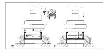
Drawn cup needle roller bearings are pressed into the housing with a mounting mandrel.
