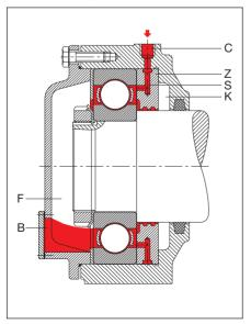
46: The grease is supplied between a bearing pair.
