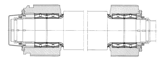
106: Roll mounting of a two-high ingot slab stand or ingot billet stand
