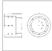
Unless otherwise specified in the shop drawing, the cylindricity tolerance should not exceed half the diameter tolerance (two-point measurement).
