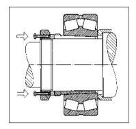
For larger bearings, considerable forces are required to tighten the nut. In such cases, the mounting nut with thrust bolts shown in Fig. 34 facilitates mounting.
