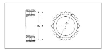
75: Diameter over rollers H<sub>a</sub> of cylindrical roller bearings NN30ASK (separable outer ring)
