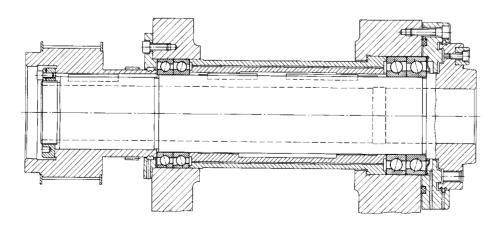
10: NC-lathe main spindle
