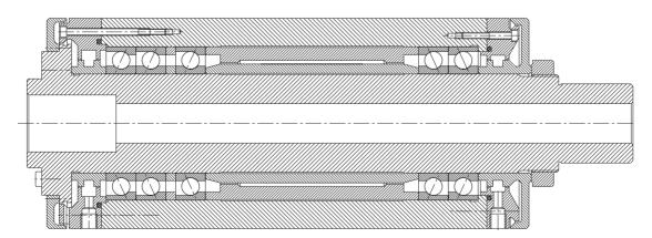
12: Drilling spindle bearing arrangement
