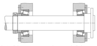
b: Spindle bearing arrangement with two tapered roller bearings in *O arrangement*. The bearings accommodate both radial and axial loads.
