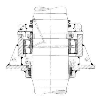
56: Rudder shaft bearing FAG RS3052KS.1.....
