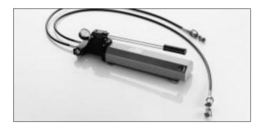
54: Hand pump set FAG 173748, consisting of a two-step piston pump (1500 bar), with 3-litre oil container, manometer, extreme pressure hose and fitting (connecting thread G 1/4)
