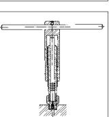
50: Larger adapter and withdrawal sleeves feature oil grooves and oil collecting grooves.
