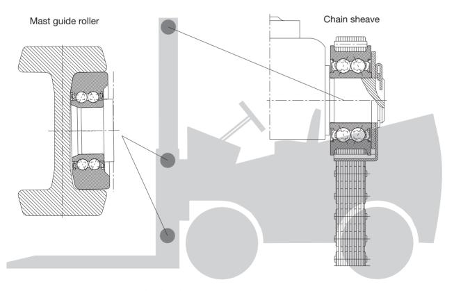
82: Mast guide roller and chain return sheave for a fork lift truck
