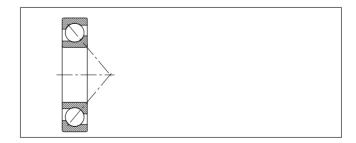
In angular contact bearings the external forces F act, not at the bearing centre, but at the pressure cone apex. This fact has to be taken into account when calculating the equivalent dynamic load P and the equivalent static load  $P_0$ .
