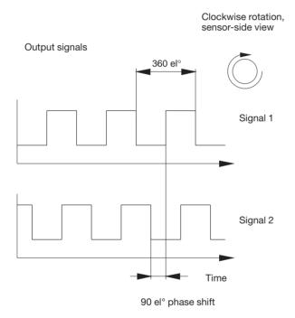
bearing inner space and sensor, the ring is provided with a flinger edge. The number of teeth on the pulse generator ring, and consequently the number of pulses per revolution, depend on the bearing size:
