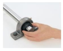
h: Series 562: tighten both threaded pins.
