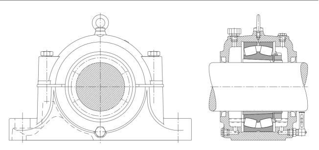
61b: Ship shaft bearing. Spherical roller bearing in S30.K housing
