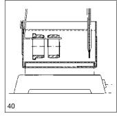
Heating cylindrical roller bearing inner rings in oil bath
