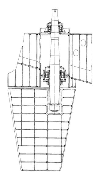
60: Spade-type rudder bearings
