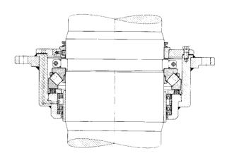
58: Rudder carrier bearing FAG RS9284N.1.....
