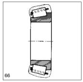
66: Pack roller/cage assembly of tapered roller bearing with grease
