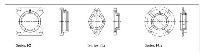
Flanged housings made from grey-cast iron (F2, FL2, FC2)
