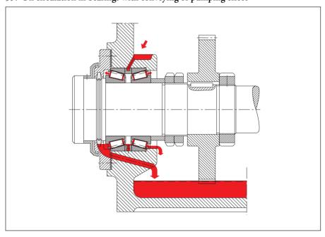
diameter. Oil is injected between the roller faces and the lip at the large raceway diameter of high-speed tapered roller bearings. This counteracts starved lubrication between lip surfaces and roller faces.
