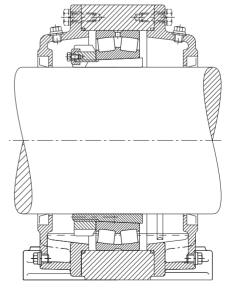
61a: Ship shaft bearing; spherical roller bearing in SUC housing
