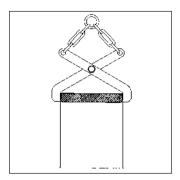
Provide for immediate axial location of mounted ring When positioning, the inner ring should be immediately held tight against the shaft shoulder, until it has cooled down to avoid any clearance between ring face and shoulder after cooling. This also applies to a pair of rings mounted side by side.
