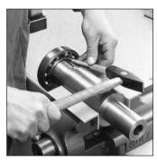
84: Provisional bearing dismounting by hammering left: wrong right: correct (use soft metal drift)
