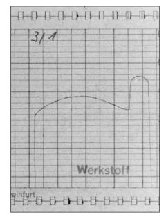
83: Cross profile chart of a worn tapered roller face
