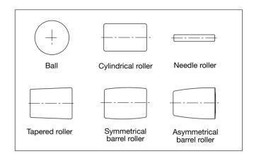
The rolling elements' function is to transmit the force acting on the bearing from one ring to the other. For a high load carrying capacity it is important that as many rolling elements as possible, which are as large as possible, are accommodated between the bearing rings. Their number and size depend on the cross section of the bearing.
