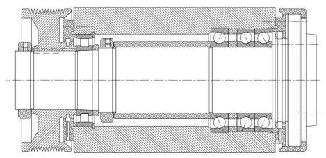
11: CNC-lathe main spindle
