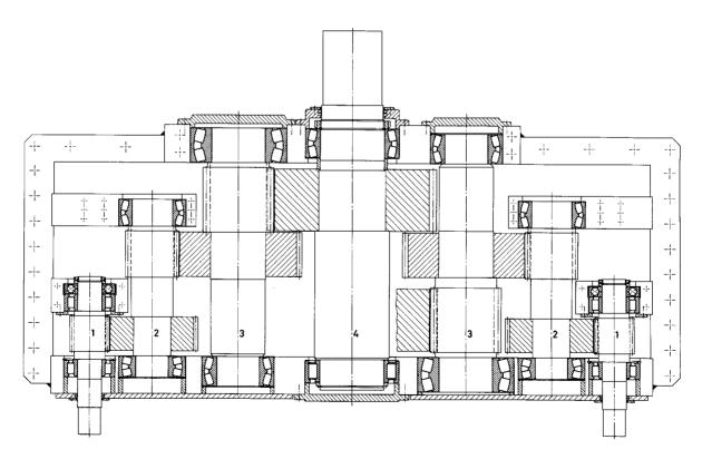
27: Spur gear transmission for a reversing rolling stand
