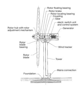
Wind energy plant, schematic drawing
