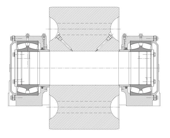
96: Support roller of a rotary kiln
