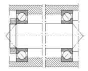
Adjusted bearing arrangement (X arrangement)
