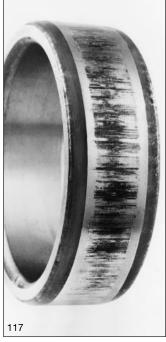
116: Indents caused by false brinelling of the raceway of a selfaligning ball bearing outer ring
