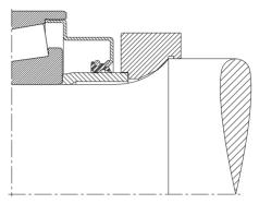
a: Rubbing radial shaft seal
