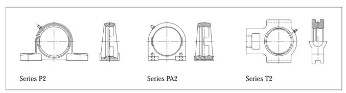
Plummer block housings (P2, PA2) and take-up unit housings (T2) made from grey-cast iron
