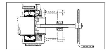
These special extracting devices are relatively complicated. They are, for example, used for applications where no oil grooves are provided in the shafts or axles for strength reasons, but which require frequent dismounting (e. g. for rail vehicles).
