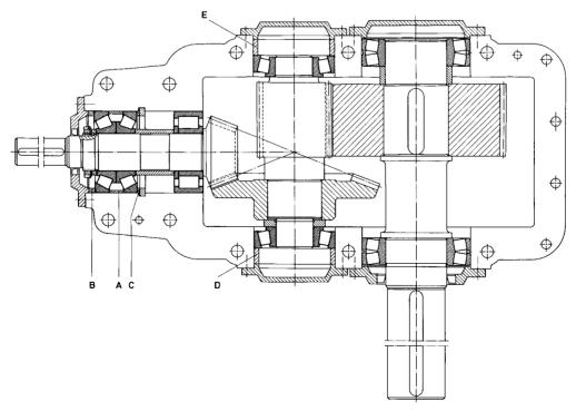
29: Bevel gear-spur gear transmission
