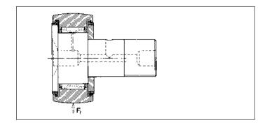
When a stud type track roller is screwed into a blind hole, the tightening torque must be applied through the slot. For this purpose, an appropriate tool is required (Fig. 26). About 75% of the tightening torques listed in the catalogues can be safely applied with these tools.
