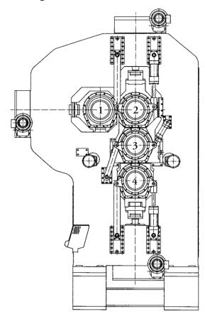
cal roller bearings (dimensions 500 x 650 x 130 mm) and deep groove ball bearings FAG 61996M.P65. At the *locating bearing* end the radially relieved deep groove ball bearing accommodates only axial guiding
