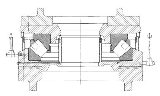
77: Crane pillar mounting with a spherical roller thrust bearing
