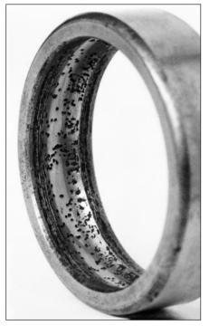
53: Corrosion of the outer ring of a deep groove ball bearing, the corrosion protection of which was destroyed by humidity
