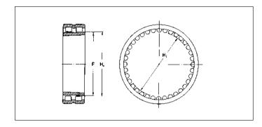
After having determined the boundary circle of the mounted outer ring roller assembly, this value is transmitted to the snap gauge. During inner ring mounting on the tapered shaft seat, the expansion of its raceway diameter is constantly checked with the aid of the snap gauge. Positive values on the dial gauge indicate preload, negative values indicate radial clearance; a zero value indicates a clearance-free bearing.
