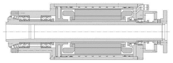
14: Motor spindle bearing arrangement of a lathe
