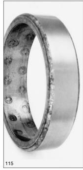
115: Corrosion marks in the raceway of a self-aligning ball bearing outer ring
