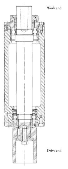
23: Vertical milling cutter spindle
