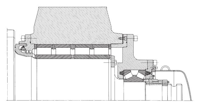
104a: Back-up roll mounting of a four-high cold rolling stand for aluminium (identical bearing arrangements at drive end and operating end)
