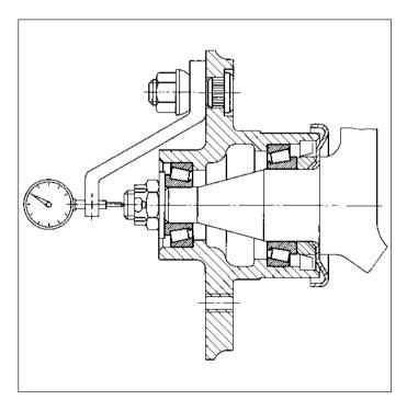
69: Measurement of axial clearance
