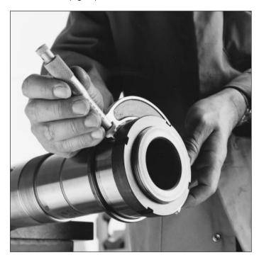
Mechanical and hydraulic equipment is available to pressfit the bearing on its tapered seat or to press a sleeve in place. Which method is the best to a given application depends on the mounting conditions.
