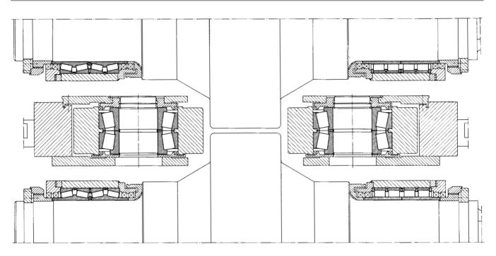
108a: Bearing mounting of horizontal rolls in the preloaded roughing stands and bearing mounting of the vertical rolls
