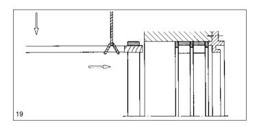
Heavy bearing outer rings with sliding fit can be mounted with a mounting lever (Fig. 19).
