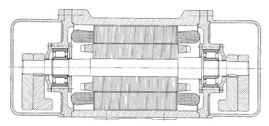
100: Imbalance rotor bearings of a vibrator motor
