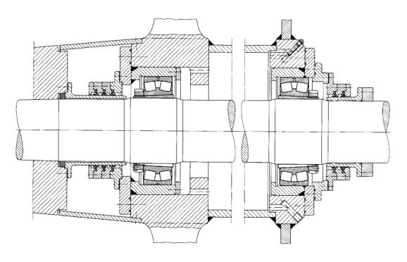
62: Stern tube or tail shaft bearing arrangement
