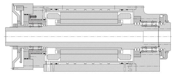
13: Bearing arrangement of a high-speed motor milling spindle
