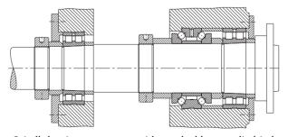
c: Spindle bearing arrangement with two double-row cylindrical roller bearings and a double-direction angular contact thrust ball bearing. Radial and axial loads are accommodated separately.
