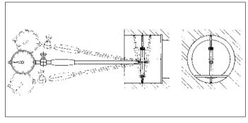
Check diameter and cylindricity of shaft and housing seats
