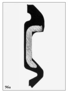
96: Cross section of a seal. a: new sealing lip; b: worn sealing lip
