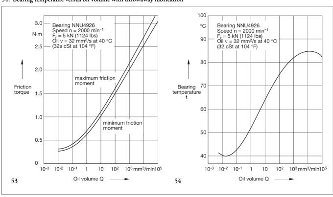
The extremely small oil quantities require an assured supply of the oil-air mixture between cage and inner ring as well as extremely accurate mating parts. The oil should have a viscosity which corresponds to the viscosity ratio  $\kappa = \nu/\nu_1 = 8$  bis 10 and contain suitable EP additives.
