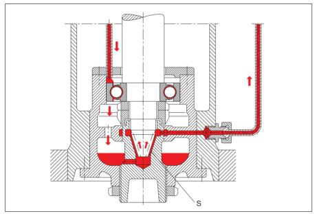
61: Oil thrown off is collected in a pocket and fed through grooves into the cylindrical roller bearing.
