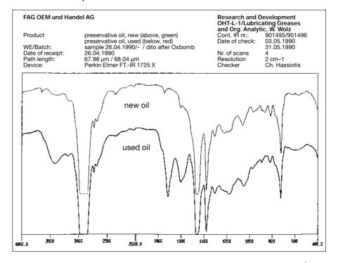
Lubricant analyses and lubricant inspections
