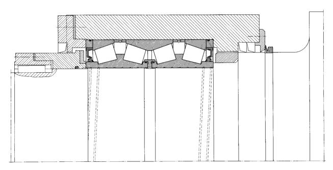
105: Work roll mounting for the finishing section of a four-high hot wide strip mill
