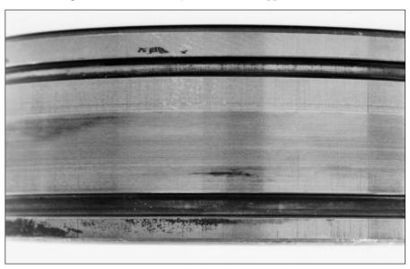
20: Lip fracture of a tapered roller bearing cone due to insufficient axial support of face
