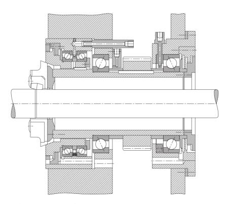
21: Bearing arrangement of a rough-turning lathe for round bars and pipes
