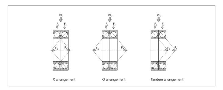
If the load carrying capacity of one single bearing is not sufficient several bearings can be mounted adjacent to one another. In this case the bearings have to be matched in such a way that as uniform a load distribution as possible and a specific clearance in the bearing set can be achieved.
