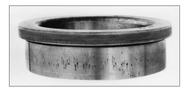
110: Premature fatigue of a cylindrical roller bearing outer ring caused by score marks visible at "a"
