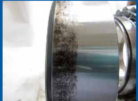
Oval deformation – Wheel hub not OK
