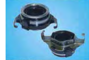
DM-0037 d 37 T58 h31 w100 Part No. 58TKZ3701 41421-49800 Application HYUNDAI
