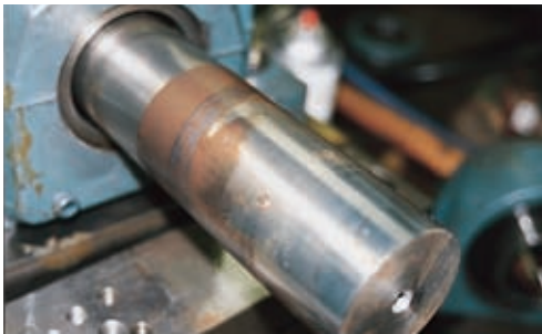
Setscrew Bearing after 500 hours
