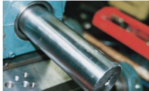
IMPERIAL bearing after 2500 hours
