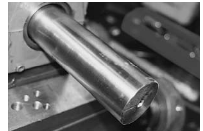
No fretting corrosion or shaft damage with the GRIP TIGHT Adapter ball bearing. Bearing is easily removed from shaft.
