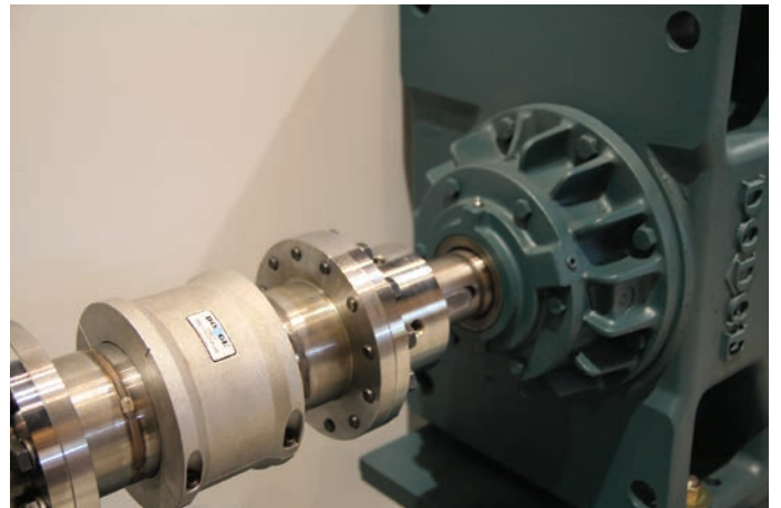
Figure 1 Dodge Grid-Lign spacer coupling mounted between a Baldor•Reliance motor and a Dodge Magnagear reducer
