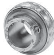
Zinc Plated Insert After Accelerated Corrosion Resistant Test
