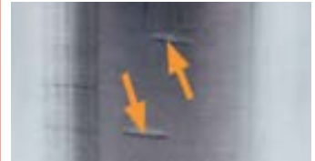
Figure 11 Raceways and rolling elements can incur indentations and nicks caused by hard, possibly sharp, objects.
