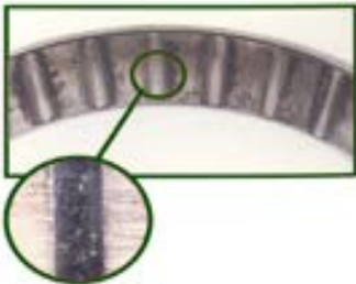
Figure 6 Localized wear spots made by rolling elements on raceway due to limited rolling/repeated impact are called false brinelling.
