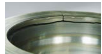
Figure 13 Thermal cracking is caused by high frictional heat due to sliding motion.
