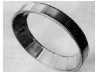
Figure 9 Plastic deformation appearance on the raceway after overloading.
