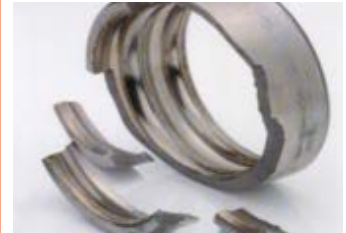
Figure 12 Forced fracture caused by a direct hammer blow.
