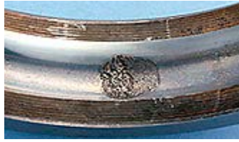
Figure 7 Electrical pitting are small burns created by arcs from improper electric grounding while the bearing is stationary
