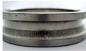
Figure 8 When electric currents pass through a bearing, there is arcing and burning at the points between the races and the rolling elements where the current jumps the air gap.
