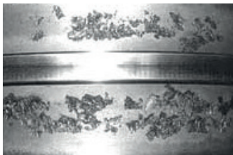
Figure 1 Fatigue spalling on the raceway
