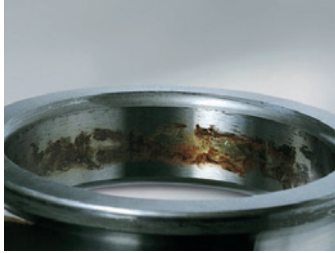
Figure 5 Fretting corrosion occurs in fit interfaces that are transmitting loads under oscillating contact surface micro-movements.
