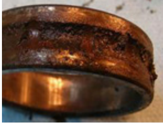
Figure 4 Rusting of a bearing inner ring caused by moisture in a lubricant.
