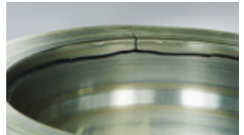
Figure 13 Thermal cracking is caused by high frictional heating due to sliding motion.
